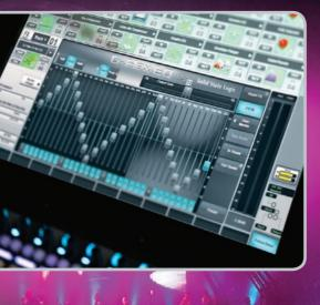
In addition to the options included in the full processing channels the effects rack offers a range of EQ options: The G-Flex EQ (which comes in 8, 16, 24 & 32 filter versions) offers incredibly flexible Graphic EQ filters. There is a 10 or 6 band Parametric with a menu of selectable filter characteristics per EQ band. There is also a smooth Contour program shaping EQ based on node selection, operated with a familiar graphic EQ user interface, allowing the creation of asymmetric EQ curves.
